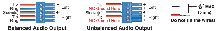
Figure 5. Audio Output Captive Screw Connector Wiring
